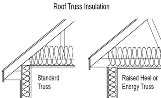
*A Raised Heel/Energy Truss provides full insulation over exterior walls resulting in energy savings and reducing the likelihood of ice damming*
